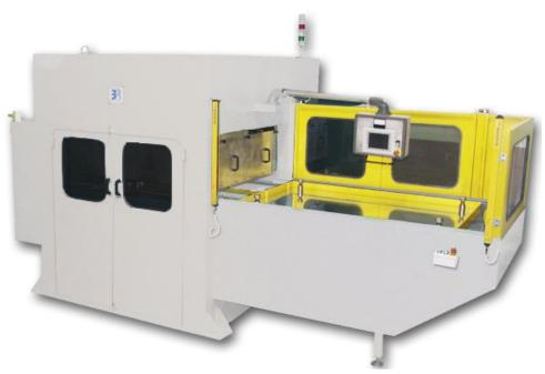
BR15 SV welding machine (with power from 8 up to 15 KW) can be designed for the HF welding of items for cars such as: sun visor, individual parts of an instrumental panel, textile insertion - HF lamination, sealing of PA structural component, reinforced-section welding on floor carpet.
