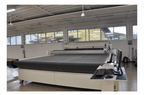
The **Plotter BR320PL** with conveyor is a versatile and high-performance machine, ideal for industrial and commercial applications that require precision and reliability. The 325 cm x 350 cm work surface allows for the processing of large materials, ensuring high production efficiency.
