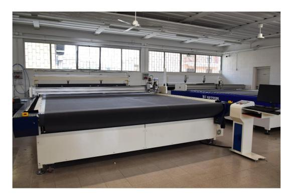
The **Plotter BR250PL** with conveyor is a versatile and high-performance machine, ideal for industrial and commercial applications that require precision and reliability. The 255 cm x 350 cm work surface allows for the processing of large materials, ensuring high production efficiency.
