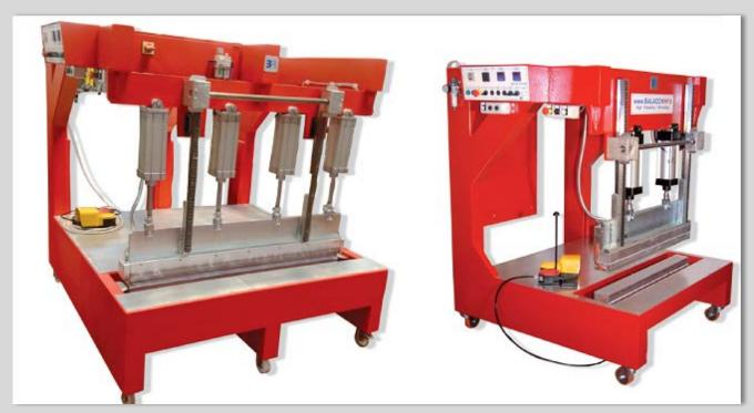
The BR10 PTFE welders are available in various size and for various purposes. This machine operates in two-step positioning mode that enables the precise placing of material and straight welding seam effectively avoiding the accidental seaming. Welding rod is usually 100x1000mm, but it could be upgraded according to client's demands. Special engraved electrodes are also available.
