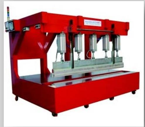
can be operated with hand or foot control. Bottom and top welding bars are separately controlled by microprocessors that permits precise temperature distribution along the both welding surfaces with maximum variation of  $\pm 1\%$ .
